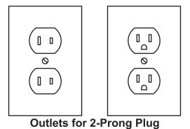
Tools marked "Double Insulated" do 1. not require grounding. They have a special double insulation system which satisfies OSHA requirements and complies with the applicable standards of Underwriters Laboratories. Inc., the Canadian Standard Association, and the National Electrical Code.
